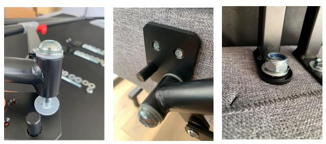
3. Insert side rail using bolt and washers (1x stainless steel washer + 1x small white plastic washer for bolt and 1x large plastic washer between bracket and rail). Two plastic washes will remain unused after assembly as spare parts.
