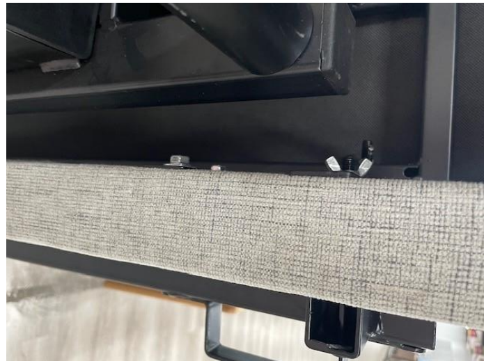
2. Please bed on the floor on FLAT position, connect transport kit to the bed end using black long bolts
