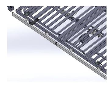
2. Connect King Single Width Extension Kit to Single bed frame using bolts and nuts supplied with the kit
